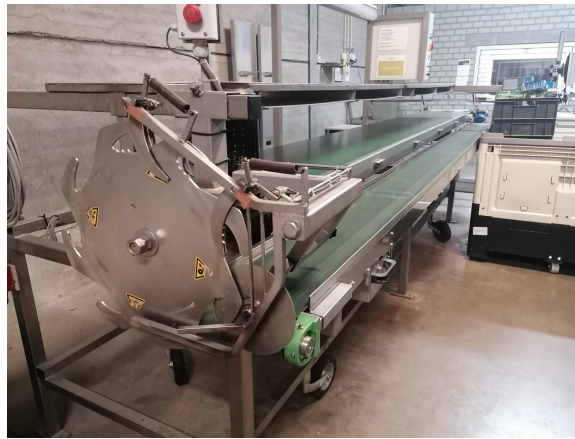
Figure 2: Current setup for root removal of chicory.
